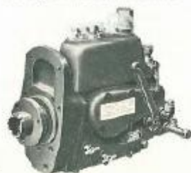
(Below) The International flange-mounted single-plunger Diesel injection pump meters and distributes the fuel in the exact quantities required by governor setting and load demands.
