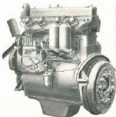
(Left) Left side of the WD-9 Diesel engine, showing the single-plunger injection pump, auxiliary and final fuel filters, water trap, and 12-inch single-plate spring-loaded clutch. Both filters have replaceable elements.
