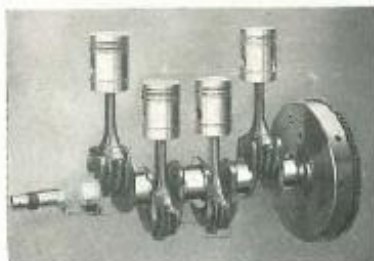
(Left) This is the crankshaft of the WD-6 engine complete with rods and pistons. Drop-forged of alloy steel, this crankshaft is precision-balanced dynamically (in motion) and statically (at rest), and is drilled for pressure lubrication, as are the connecting rods.
