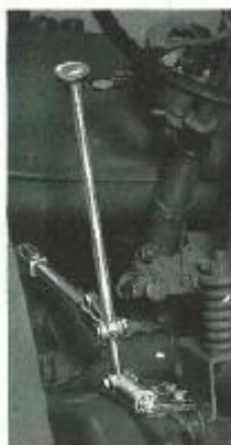
This "remote control" gear shift attachment, available for factory or field application on W-9 and WD-9 tractors, facilitates gear shifting on these large models.
