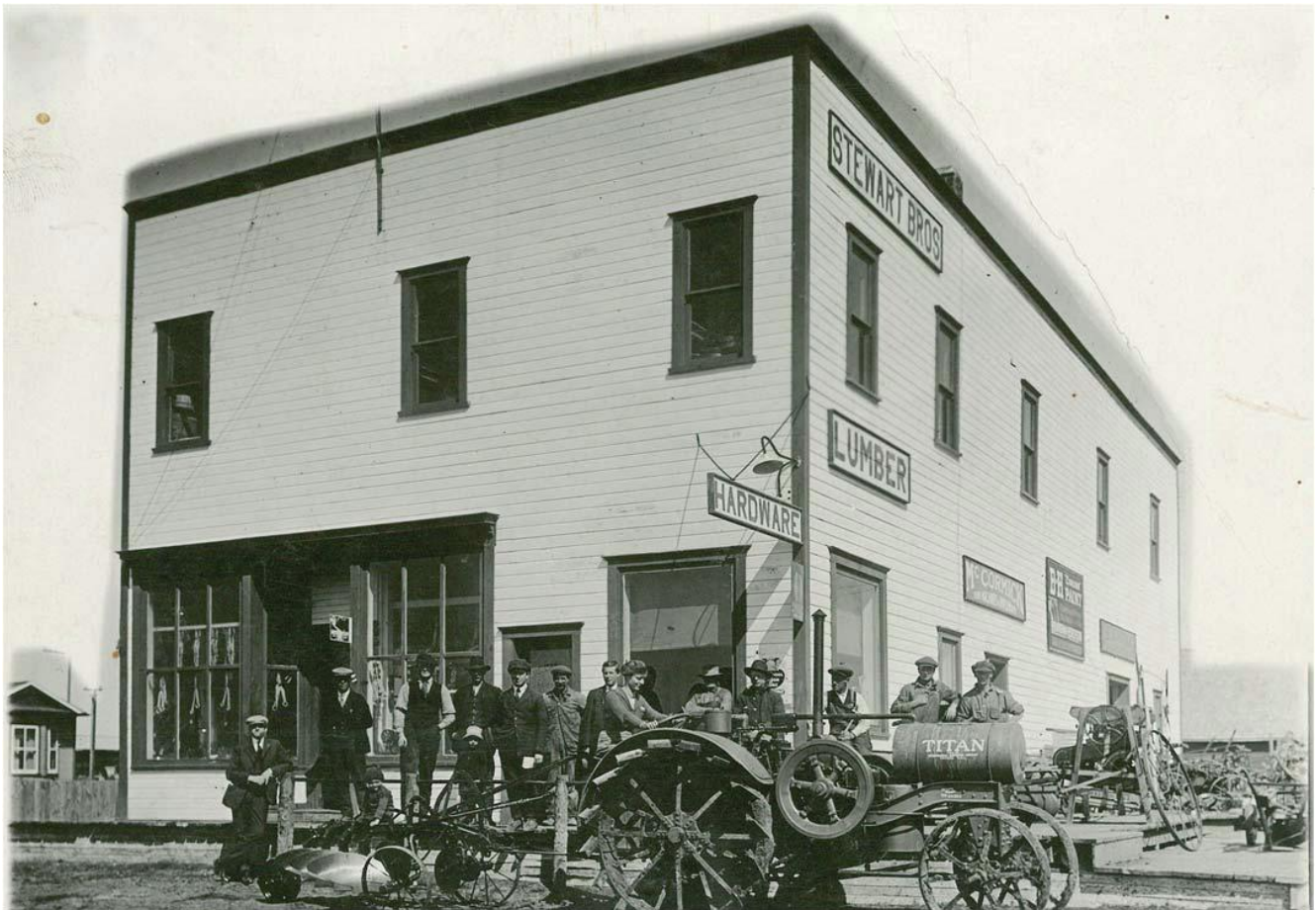
The Stewart Brothers Penhold store and staff in 1921. Norman, wearing a cap, is standing in the doorway while Tom is at the corner of the store standing behind the exhaust of the Titan tractor. In the foreground is a TITAN tractor S.N. 40529, circa 1919. Between 1915 and 1922, 78,464 of these horizontal two-cylinder chain-drive tractors were built.
