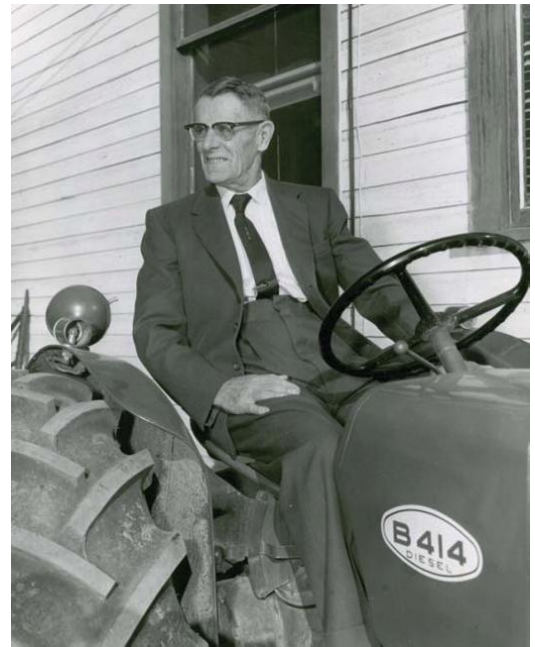
Tom Stewart seated on a British-built IHC B-414 diesel tractor, circa 1964. When the B-414 tractor was launched in 1961, IHC advertising literature described it as "The tractor with everything you've wanted most". The B-414 was powered by a 36 h.p. diesel engine, transmission was via an eight forward and two reverse speed gearbox.
