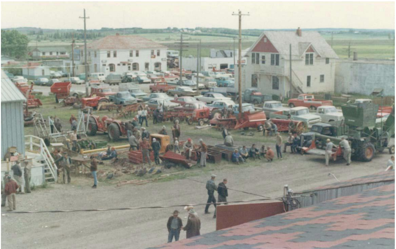
This photo of the 1968 machinery auction was taken from the roof of the Penhold store's then-new arch rafter building supply storage shed. Worth noting are the two WD9 tractors joined with a tandem hitch, seen to the right of the platform warehouse. This was a farmer innovation to get more horsepower and traction. They went out of style quickly once machine companies came up with their own versions which were more compact and had a much tighter turning radius.
