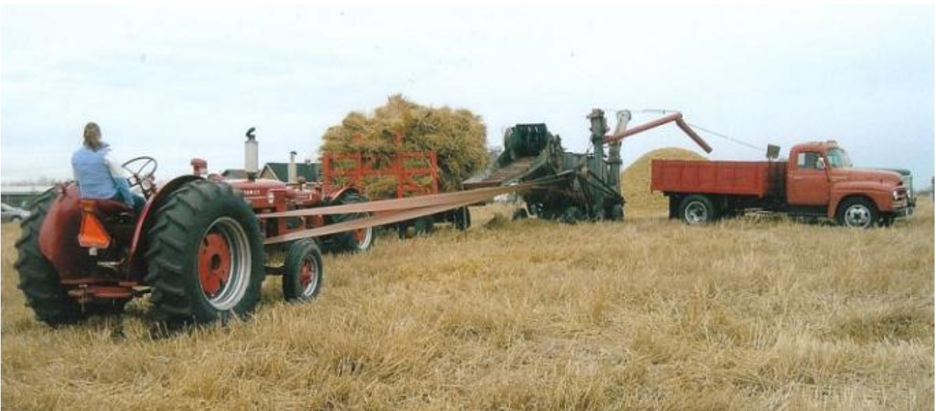
Here's the McCormick Super WD 9 on the belt. A 28 inch McCormick thresher, R150 International grain truck, in behind is the KB7 International and Super W4 hauling bundles in from the field.
